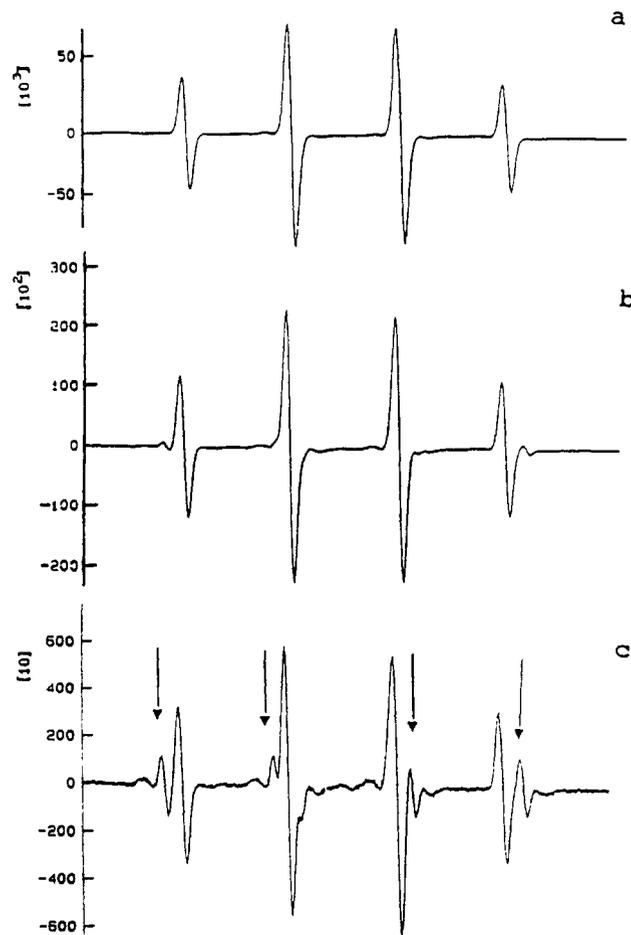
**Figure 1.** EPR spectra of (a) 5 mM  $\text{H}_2\text{O}_2$ , 5 mM  $\text{FeSO}_4$ , and 100 nM DMPO in 0.1 M phosphate buffer (pH 7.4); (b) as in (a) but with 10 mM carnosine; (c) as in (a) but with 25 mM carnosine.
