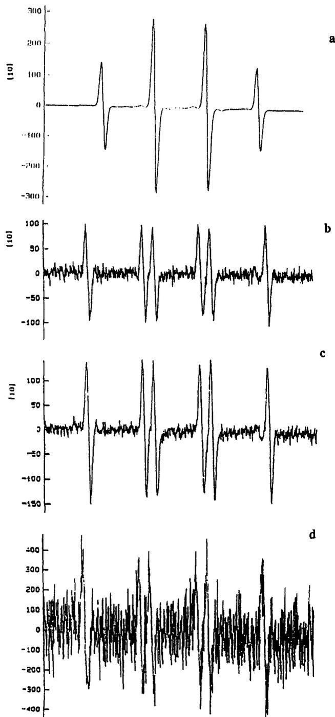
**Figure 2.** EPR spectra of (a) 5 mM  $\text{H}_2\text{O}_2$ , 5 mM  $\text{FeSO}_4$ , and 10 mM DMPO in 0.1 M phosphate buffer (pH 7.4); (b) as in (a) but with 25 mM carnosine; (c) as in (a) but with 25 mM Gly-His; (d) as in (a) but with 25 mM homocarnosine.
