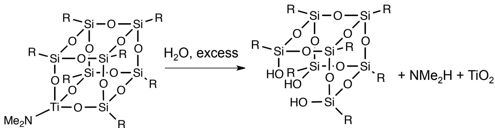
Ti-POSS reaction with water results in Ti leaching (loss) from the active catalysts
