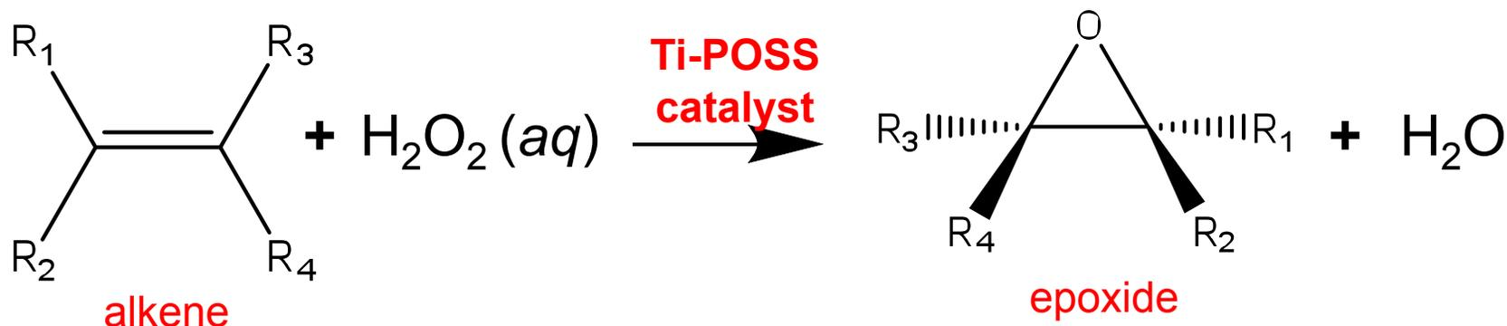
**Hypothesis:** enclosing Ti-POSS catalysts in a hydrophobic (water-excluding) environment would keep water out while allowing in the alkene and H<sub>2</sub>O<sub>2</sub>; thus, permitting alkene epoxidation to occur
