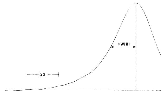
Fig. 1. Half-width at half-height of the  $M_1 = +1$  low-field EPR line of 5-NS in intact erythrocytes. EPR spectrometer conditions are indicated in the text.
